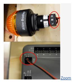
Requires: Wire stripper, 2 pin cable, Robot Signal Light, 18AWG red wire, very small flat screwdriver
