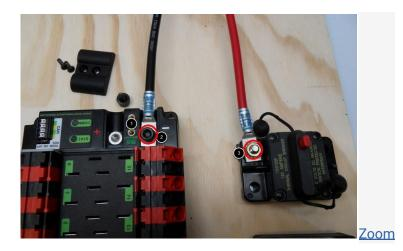
Requires: Battery Connector, 6AWG terminal lugs, 1/16" Allen, 5mm Allen, 7/16" Box end
